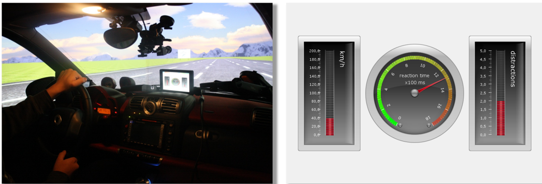
Figure 12.1: Reaction time estimated by speed and visual distraction displayed in the car.
